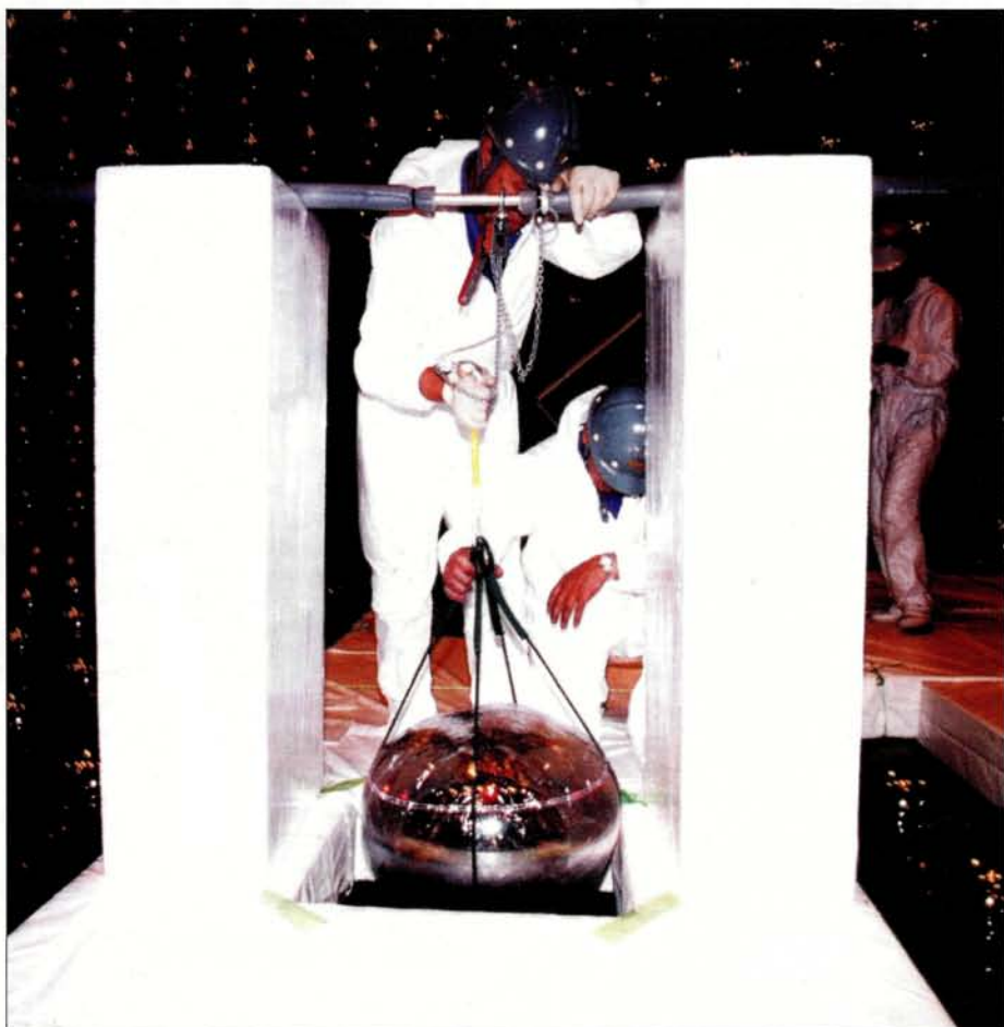
Routine maintenance at Super-Kamiokande, showing the size of the photomultiplier.
