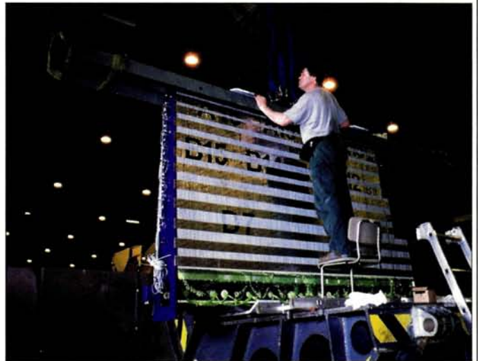
Fabrication at JINR Dubna of a "tile" calorimeter module for the ATLAS experiment at CERN's Large Hadron Collider. Each of the 64 modules weighs 20 tonnes. JINR also coordinates work for other major modules at both the ATLAS and CMS experiments.
