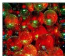
"Random" laser. The spaces between the spheres of glass are filled with laser dye dissolved in a liquid crystal. (D Wiersma.)
