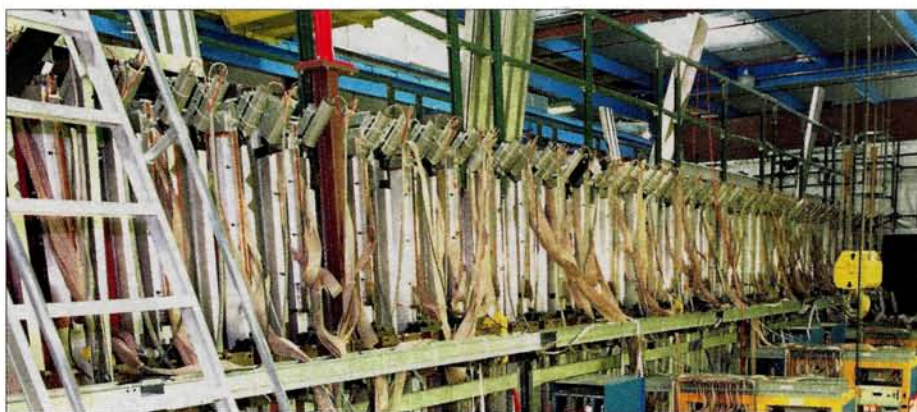
View of the NuTeV neutrino detector at the Fermilab Tevatron, which used a 700 tonne sandwich of steel target plates interspersed with drift chambers and scintillators.
